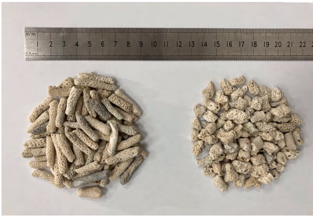
Fig. 1. Photograph of two representative types, namely stick-like and lump-like, of coral sand particles.
