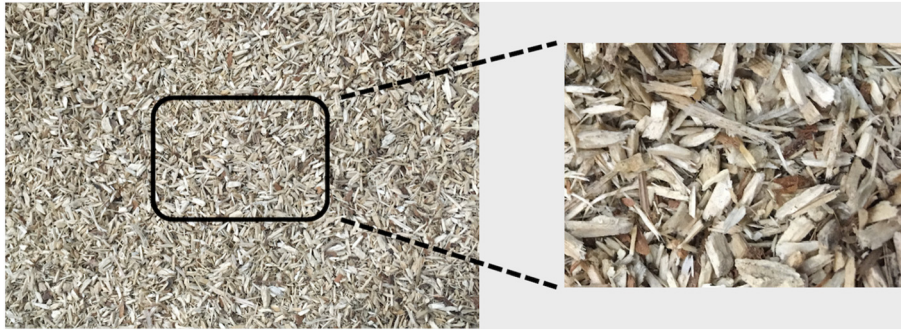
Fig. 1. Loblolly pine forest residues after being hammermilled with a 25 mm screen.
